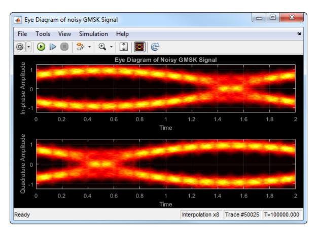
Observe that vertical striping is present in the eye diagram. This striping is the result of input interpolation, which has limited accuracy in low-SNR conditions.
