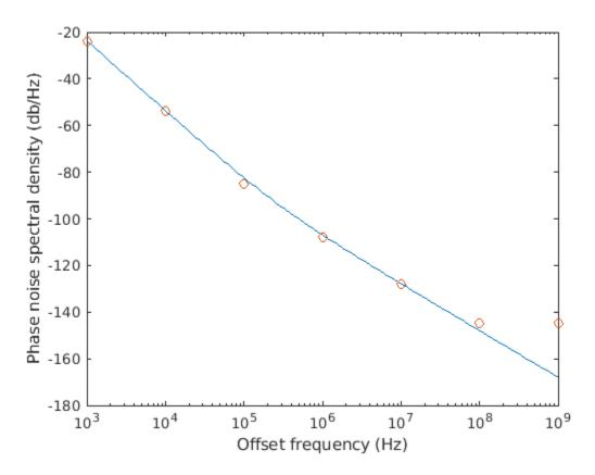
It appears that there is a measurement noise floor at -140 dBc/Hz for the specification dataset, and the phase noise for the device under test is probably below that noise floor for offset frequencies above 100 MHz. In this case, a set of parameter values that fit best to the data at lower frequency offsets is likely to produce a more accurate model.
